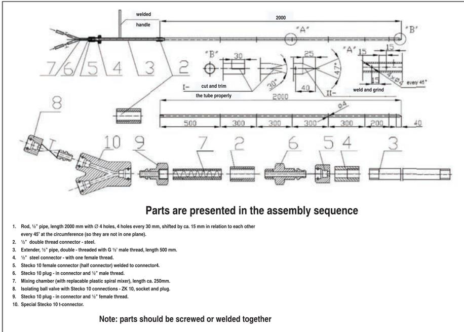
**Figure 3: 1/2" Rods and Injection Accessories**
