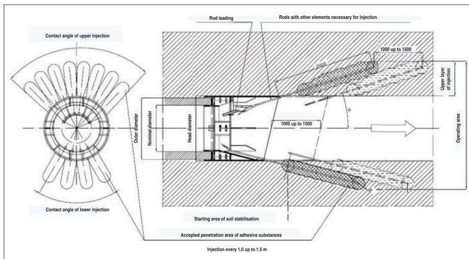
Figure 2: Spacing of Holes and Operating Area of Adhesive Substances on Soil.
