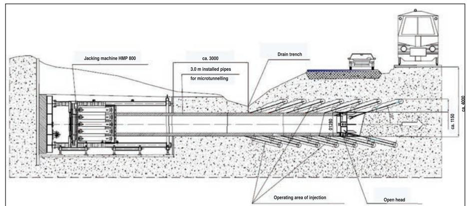
Figure 1: Jacking Under a Traffic Object with Use of Soil Stabilization Technology by Injection and Penetration of Multi-Component Glues.
