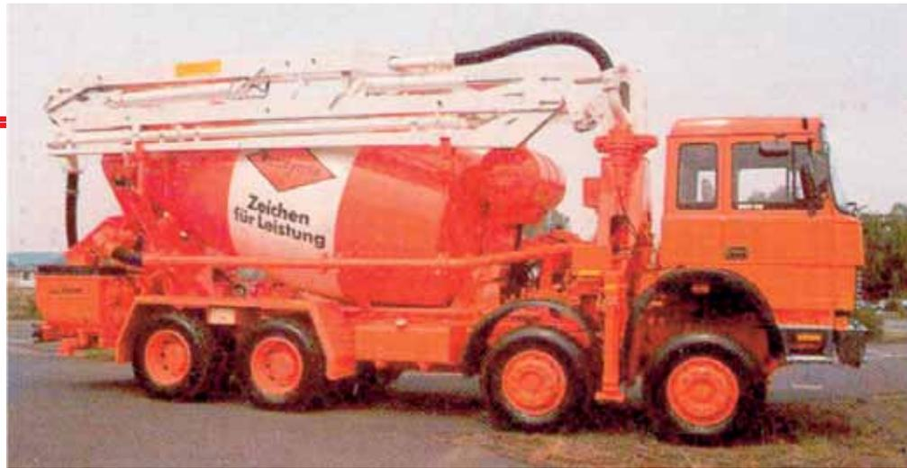
**Figure 4** - Truck mixer with concrete pump and distributing boom.
